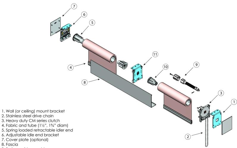
5. Spring loaded retractable idler end
